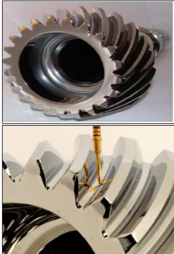
**Figure 9. TTO Bevel Pinion Post MMP Treatment**
