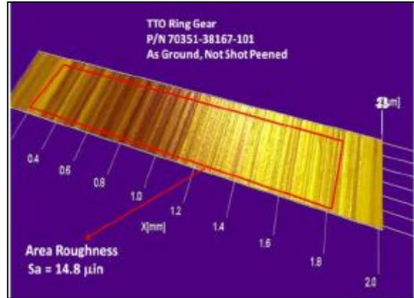
Figure 25. Surface Roughness and Topography of TTO Gear Prior to Testing
