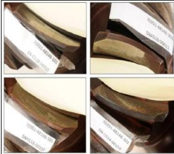
**Figure 5. Driving Tooth Surfaces of Candidate Pinions**
