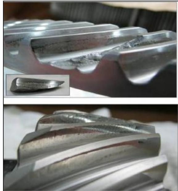
**Figure 3. TTO Bevel Gear and Pinion post Block I Overload Testing**
