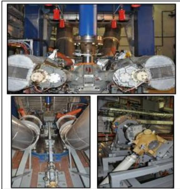
Figure18. HeDS Facility with Test Gearboxes Installed
