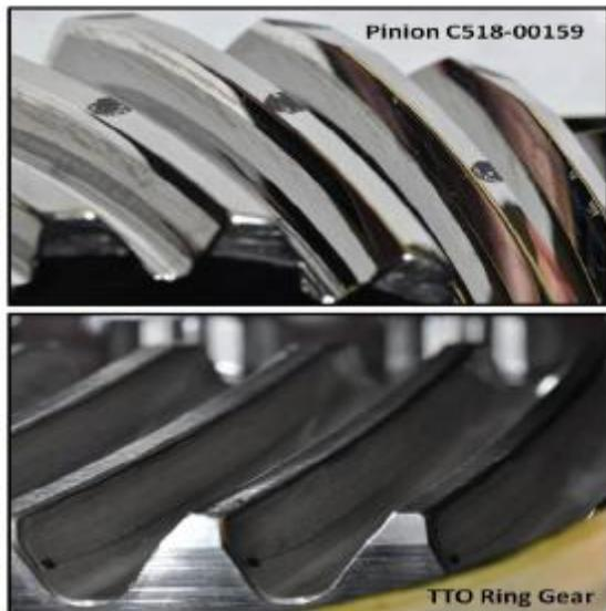
**Figure 19. Post Test TTO Pinion and Bevel Gear Gear Tooth Finish and Topography Changes During Testing**
