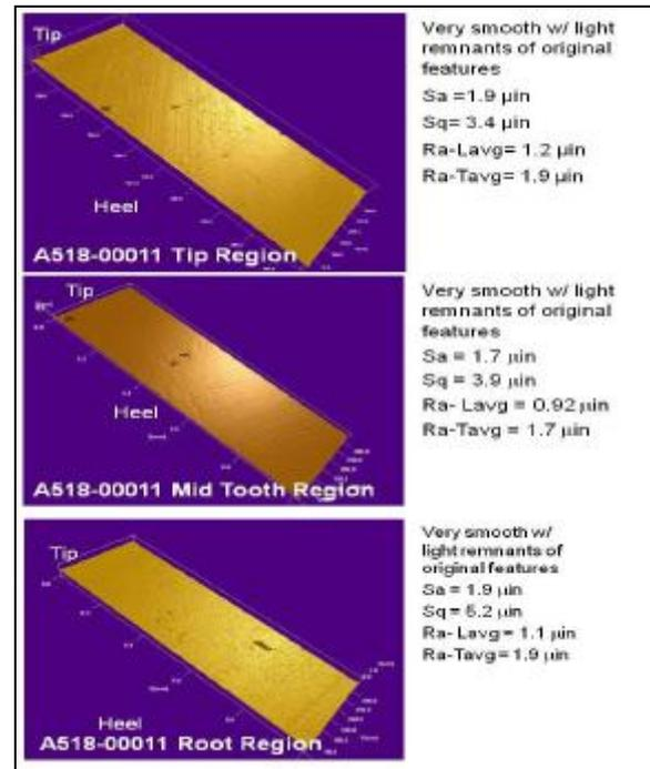
**Figure 15. Pinion A518-00011 Post MMP Surface Finish and Topography Characteristics**
